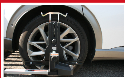
8 sensors allows measurement of rear set back
