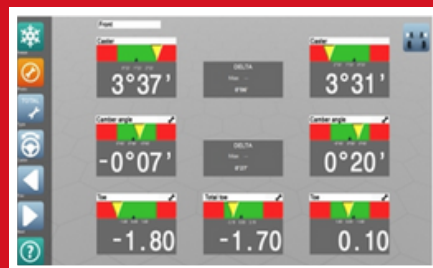
Live simultaneous readings of castor, camber and toe
